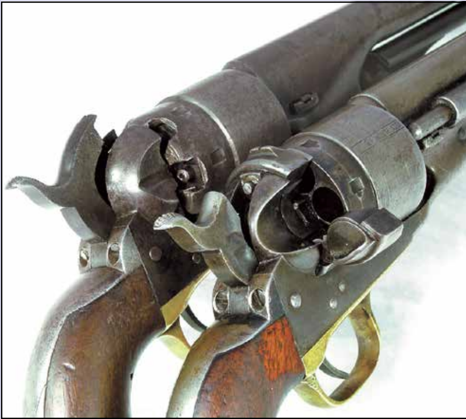
.44 RICHARDS (TYPE I) BREECH COMPARED TO 1860 ARMY
