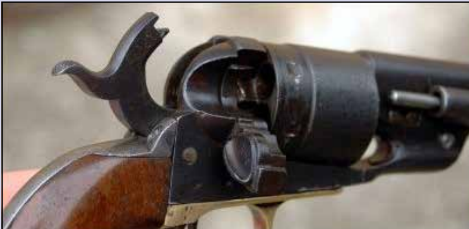
.44 RICHARDS TYPE II (TRANSITIONAL) BREECH AND HAMMER MOUNTED FIRING PIN
