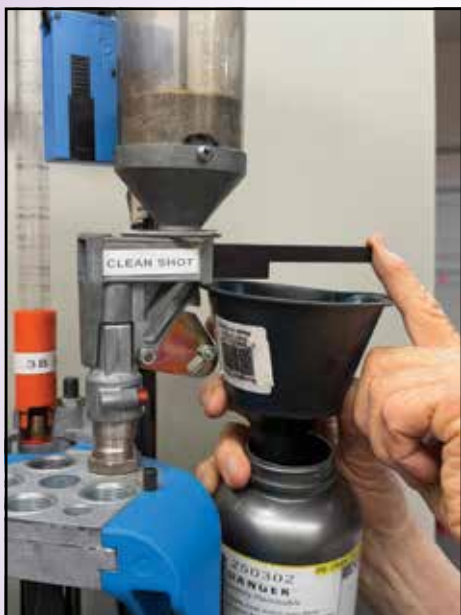
THE DRAIN-N-CHANGE ENABLES DRAINING THE DILLON POWDER MEASURE WITHOUT REMOVING IT FROM ITS MOUNT. THIS IS THE CLOSED POSITION.
