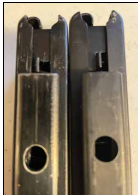
L-R: ORIGINAL SUBMACHINE GUN 30-ROUND MAGAZINE WITH 1/4-INCH MODIFICATION VS. T-RIFLE 30-ROUND MAGAZINE.
