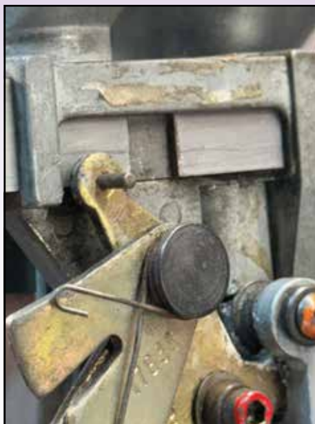
THE ONLY TRICKY PART IS REMOVING AND REPLACING THE BELL CRANK CUBE WITHOUT LOSING IT.
