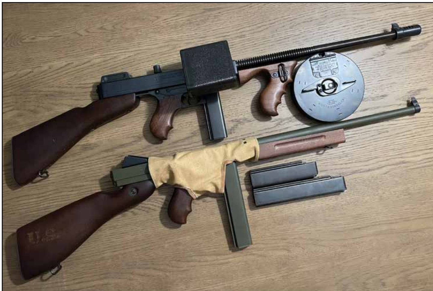
TOP: M-1927A-1 WITH BRASS CATCHER, 50-ROUND DRUM, AND STICK MAG. BOTTOM: M-1942A-1 WITH ACTION COVER, 30- AND 20-ROUND MAGS.
