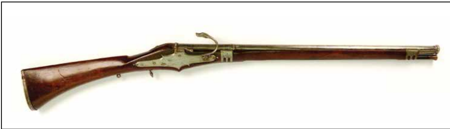
LATE MATCHLOCK, SPANISH OR ITALIAN, CIRCA 1580-1600, WITH A .65-CALIBER ROUND/OCTAGON BARREL 25-7/8" LONG, AND DECORATIVE INLAYS IN THE STOCK. THIS PIECE HAS A CONVENTIONAL TRIGGER INSTEAD OF THE TILLER-LIKE TRIGGER OF EARLIER ARMS, AND A WIDE LOCKPLATE SUGGESTIVE OF THOSE USED ON WHEELLOCKS.
