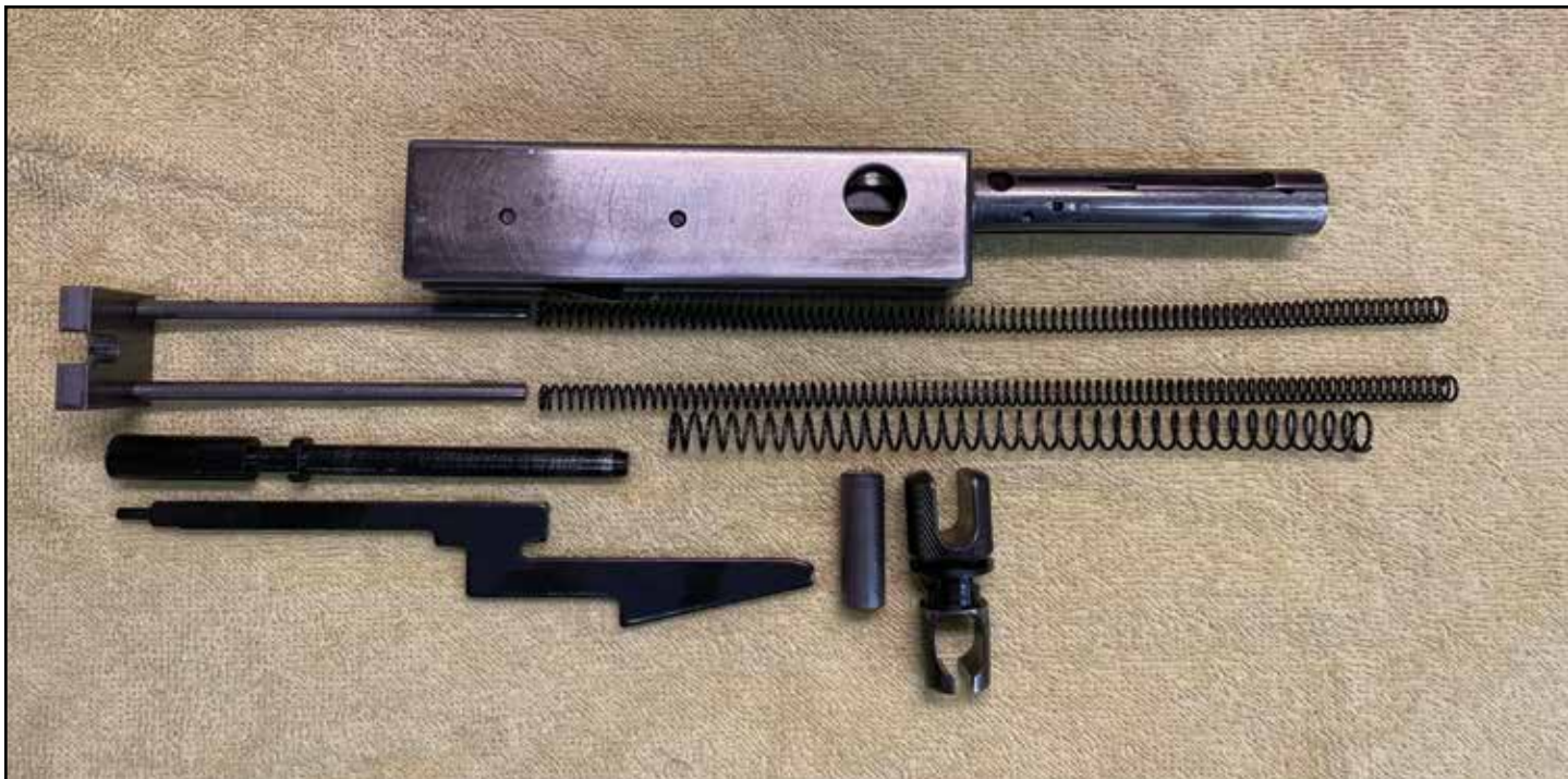
UPPER ACTION PARTS — BOLT BLOCK, RECOIL SPRING GUIDE WITH SPRINGS, FIRING PIN ROD AND SPRING, PIN, HAMMER AND CHARGING HANDLE.
