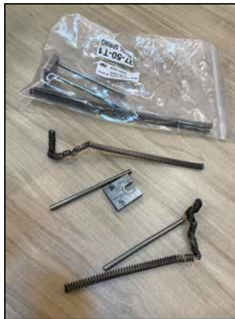
A BROKEN RECOIL SPRING GUIDE WITH DAMAGED SPRINGS AND THE BROKEN FIRING PIN.
