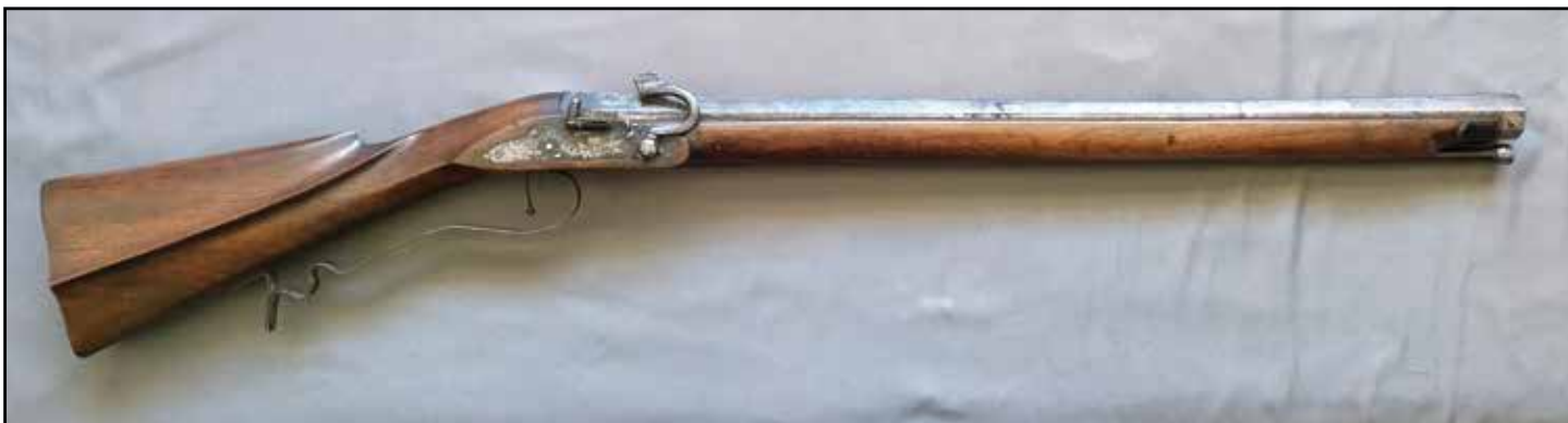
LATE MATCHLOCK, CIRCA 1580-1600 WITH A .54-CALIBER OCTAGON BARREL 23" LONG. THIS PIECE ALSO SHOWS FEATURES TYPICAL OF WHEELLOCK ARMS, SUCH AS THE TRIGGER, THE LONG RECURVED TRIGGER GUARD, AND THE CONTOURS OF THE BUTTSTOCK.
