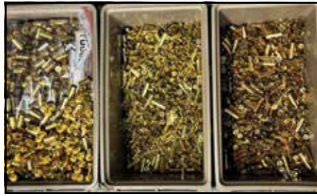
THE .45 ACP ON THE LEFT IS MULTIPLE VINTAGES. THE BAG IS TWO YEARS OLD. THE REST IS FRESH, BRASS JUICE, STRAT-O-SHEEN AND ONE SHOT. THE .38 SPECIAL IN THE MIDDLE IS 16 MONTHS OLD. BRASS JUICE, STRAT-O-SHEEN, AND ONE SHOT. THE .38 ON THE RIGHT WAS THE SAME BUT NO ONE SHOT AND NO PINS.
