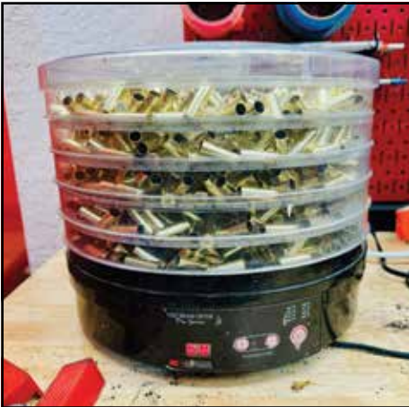
A 10-YEAR-OLD BRASS DRYER. NO TIMER. GET ONE WITH A TIMER IF YOU CAN.
