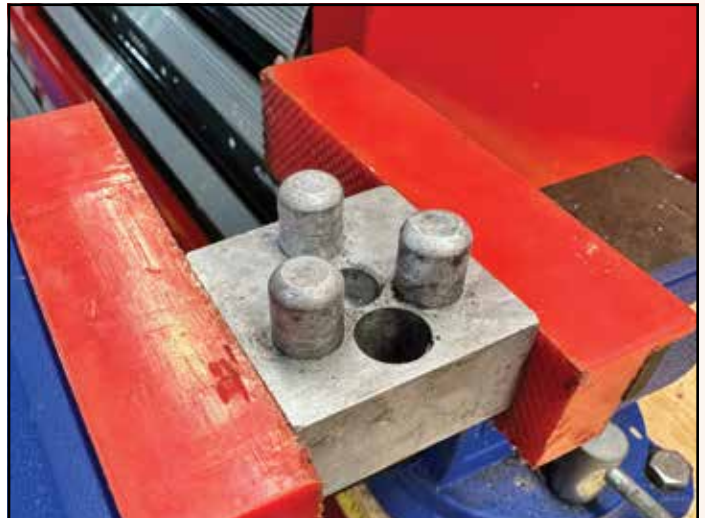
FROM KINGSNAKE, A STAND FOR A PERCUSSION PISTOL. THIS ONE IS FOR A RUGER OLD ARMY. IT STABILIZES THE CYLINDER FOR WORKING ON THE NIPPLES. THE HOLE IS FOR CLEARING STUCK BALLS.
