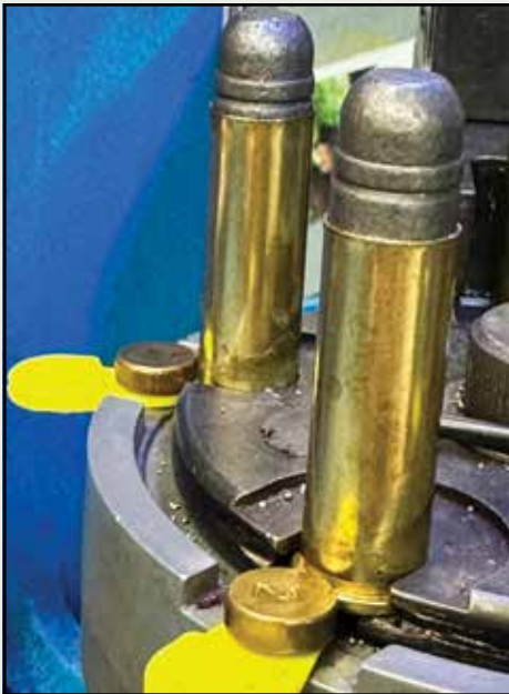
IN LINE ON A DILLON XL750. THE BULLETS ALL LOADED WITHOUT ANY BLEMISHES. CRIMPING ON THE CRIMP GROOVE IS RECOMMENDED.
