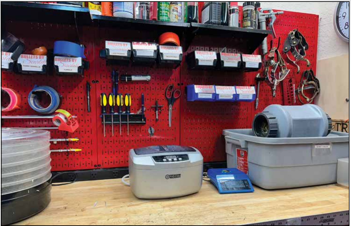
THE BRASS PREPARATION PART OF MY SHOP. THE 10-YEAR-OLD BRASS DRYER ON LEFT. ON THE RIGHT IS A TUB WITH THE FRANKFURT ARSENAL ROTARY TUMBLER IN IT. LEAKS FROM THE LIDS HAPPEN, SO I DO NOTHING WITH THE WET TUMBLER UNLESS IT'S IN A TUB OR A SINK.
