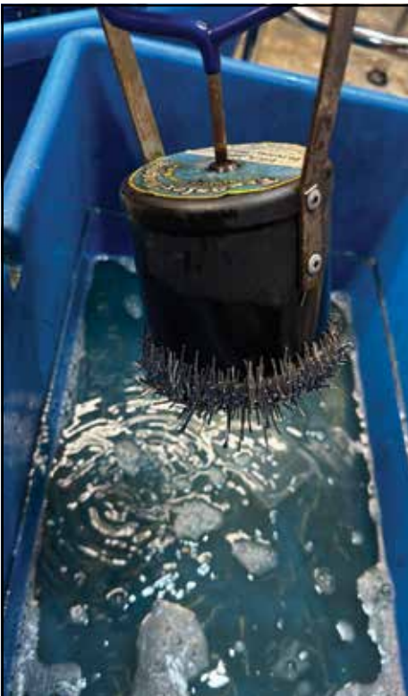
USING A FRANKFORD ARSENAL PICK UP MAGNET TO RETRIEVE PINS. DON'T USE PINS WITHOUT ONE.
