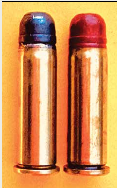
NEXT TO A 158-GRAIN RNFP HI-TEK COATED BULLETS BY SCARLETT, THE PROCAST BULLET MATCHED MOST DIMENSIONS, EXCEPT FOR WEIGHT. IT FED IN A '73 JUST AS SMOOTHLY.
