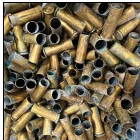
TYPICAL BLACK POWDER BRASS WITH NO PRE-SOAKING. THIS IS TOUGHER THAN SMOKELESS BRASS.
