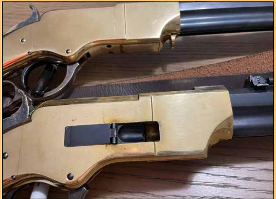
rel-magazine system yet is charged like the Model 1866 Improved Winchester via a hinged-mounted door-to-open on the rifle frame's right side. My rifle was manufactured by Uberti in 2004 and imported by Taylor's and Co. according
