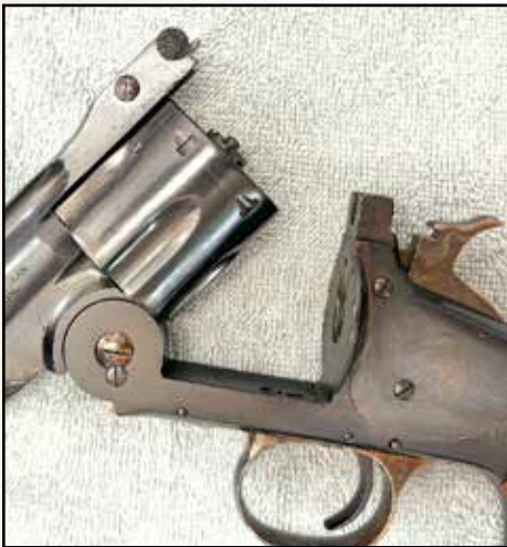
NO. 3 LOCK UP TOP STRAP AND HAMMER NOTCH (AUTHOR PHOTO).
