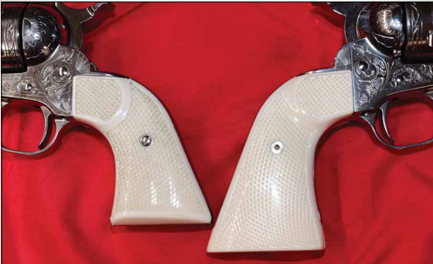
STANDARD GRIP ON THE LEFT, 1860 ON THE RIGHT. IF YOUR LITTLE FINGER GOES UNDER THE STANDARD GRIPS THE 1860S WILL GIVE YOU A BETTER GRIP.
