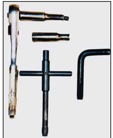
RUGER COMBINATION 3/16" SOCKET NIPPLE WRENCH AND SCREWDRIVER FOR LOCKING AND UNLOCKING THE BASE PIN; CRAFTSMAN 1/4" DRIVE WRENCH WITH 1/4" DEEP SOCKET AND ONE MODIFIED BY KINGSSNAKE TO FIT STANDARD NIPPLES; SLIX WRENCH FOR NIPPLES.
