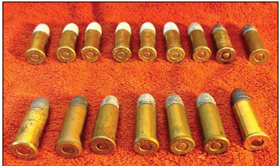
TOP ROW — .44 S&W (AMERICAN) AMMUNITION BASE VIEW BOTTOM ROW — .44 S&W RUSSIAN AMMUNITION BASE VIEW — FROM AUTHOR'S COLLECTION
