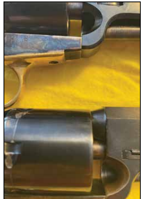
PIETTA FACTORY FRAME PORT VS. THE BOTTOM PORT, SLIGHTLY MODIFIED BY HAND BY THE AUTHOR.
