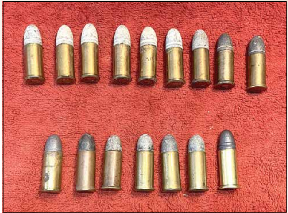
TOP ROW — .44 S&W (AMERICAN) AMMUNITION SIDE VIEW BOTTOM ROW — .44 S&W RUSSIAN AMMUNITION SIDE VIEW
