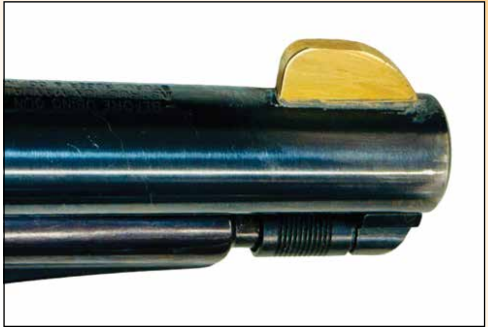
ON TARGET BRASS FRONT SIGHT GOES OVER THE TOP OF THE STANDARD SIGHT. THIS ONE HAS BEEN FILED FOR ZERO.
