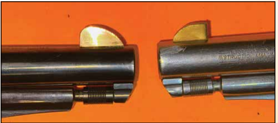
ON LEFT IS THE ON TARGET FRONT SIGHT. ON THE RIGHT IS THE SURE HIT FRONT SIGHT.
