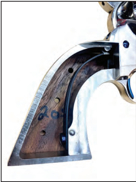
FLAT MAINSPRING. THE ACTION IS PURE 1873 SAA.
