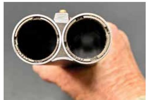
THE 20" BARRELS HAVE REM-CHOKE REMOVABLE CHOKE TUBES. FIVE ARE INCLUDED.
