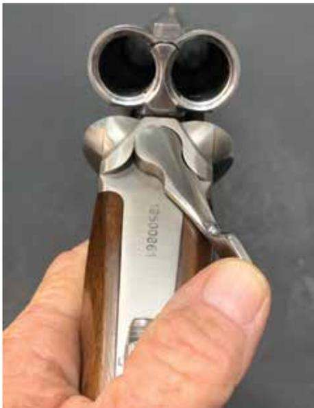
THE POINT OF LEVER MOVEMENT WHEN THE BARREL OPENS. THIS IS EASIER TO USE THAN THE STOCK POSITION EVEN IF YOU'RE LEFT-HANDED.
