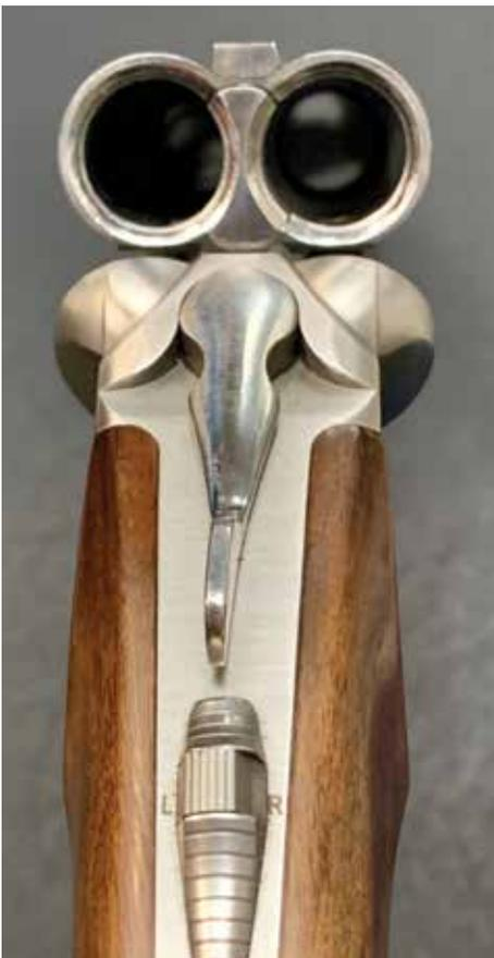
IMPROVED LEVER IN STOCK LOCATION. BARREL SELECTOR SWITCH IS ON THE MANUAL SAFETY.
