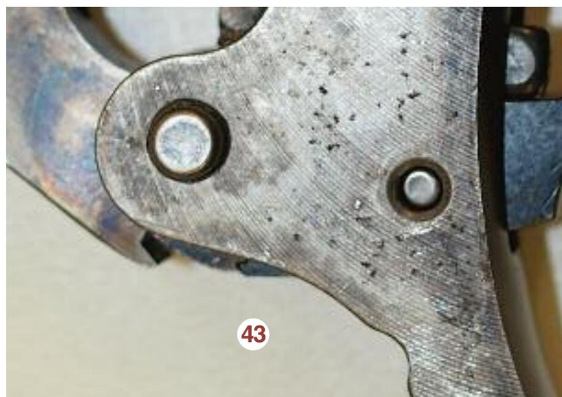
two trigger screws on the front of the trigger become visible. **Photo 42.** Insert the Allen wrench into the UPPER screw and adjust sear engagement. **Photo 43** shows the sear fully engaged in the full cock notch.
