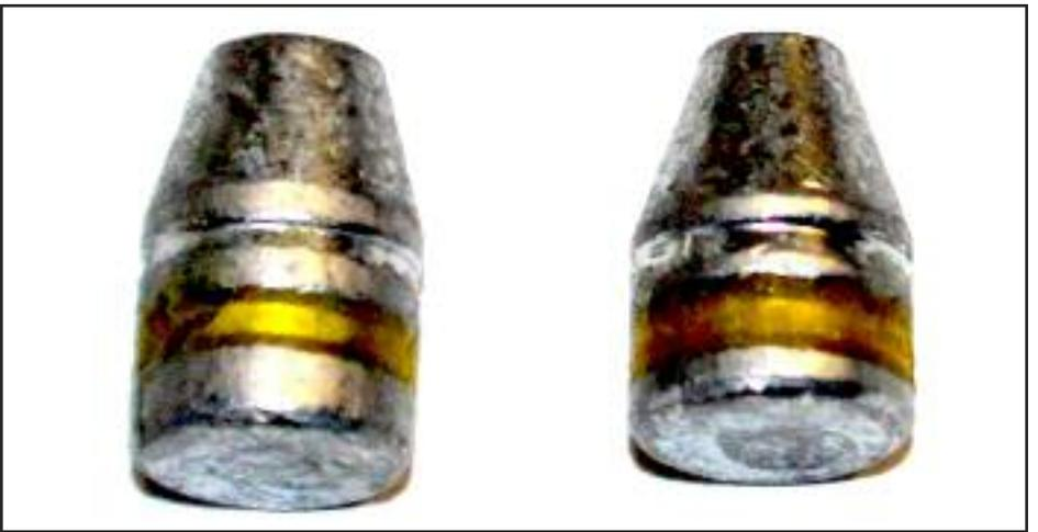
*Two popular .38/.357 bullets for Cowboy Action Shooting™. On the left is the 125-grain TCFP. It worked very well in the test. On the right is the 105-grain TCFP. It worked very well with American Pioneer Powder but not so well with Goex Cartridge.*
