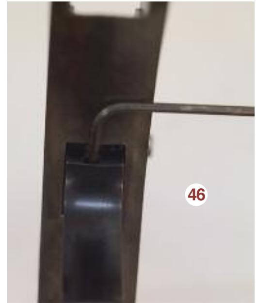
push in the safety bar and pull the trigger until the lower adjusting screw is visible in the front of the trigger. **Photo 45.** Insert the Allen wrench (try using the short end of the Allen wrench as it provides more clearance for this screw) and adjust the forward travel of the trigger. **Photo 46.** You want to adjust the trigger so that when the trigger is pulled the sear tip just
