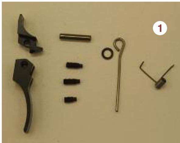
new trigger pivot pin and three adjustment screws; a trigger spring spacer and trigger spring; and a new safety lever spring. Aside from a quality set of hollow ground gun screwdrivers
