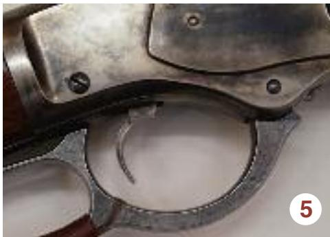
used a two-piece trigger, with the sear being able to pivot independently from the trigger. This creates a problem for speed tuning a modern 73 for SASS competition. **Photo 5** shows the trigger at its rearward
