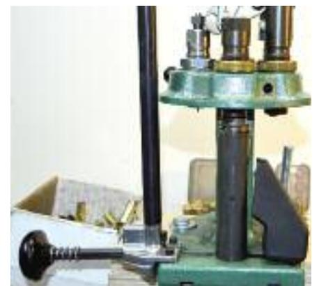
*... unless you want to full-length resize the completed round at station 5, using the RCBS Cowboy sizing die with the de-capping mechanism removed.*
