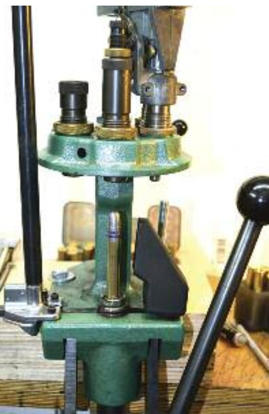
*Round is at station 4, ready for bullet seating. When the bullet is seated at station 4, the round is complete—unless ...*
