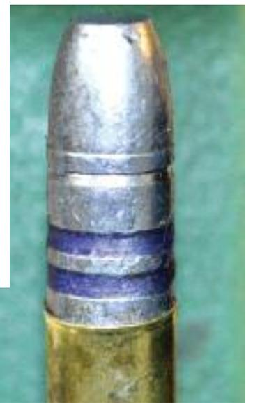
*Flat-based bullets will work best if the case is slightly belled at station 2, the expander die.*
