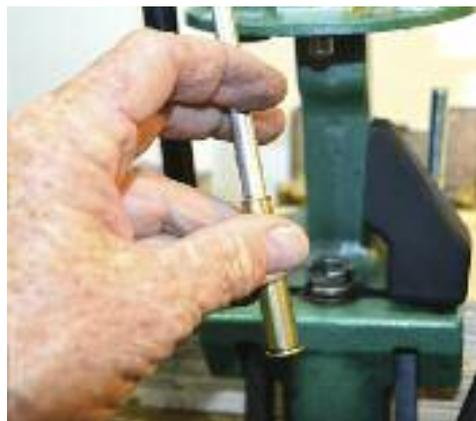
*You can measure the powder level with a flat-bottomed rod or dowel probe with a mark on the side for the correct depth. In this case, the mark coincided with the length of the bullet to the crimp groove.*
