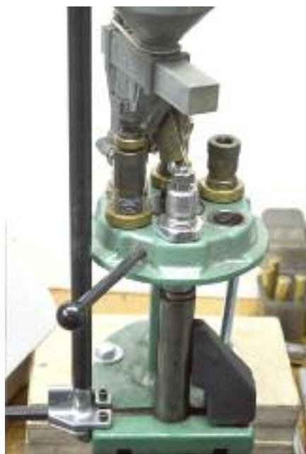
*I use five of the six die mounting holes in the RCBS Turret Press—(1) Lee De-capping/resizing die, (2) RCBS Cowboy expander die with the large expander plug, (3) Dillon Powder measure die, (4) RCBS Cowboy seating/rimp die, (5) RCBS Cowboy de-capping/resizing die with de-capping mechanism removed to resize completed round.*
