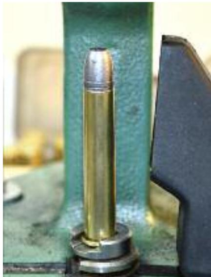
*The resulting round has any bulges removed, making it less likely to stick in the chamber.*
