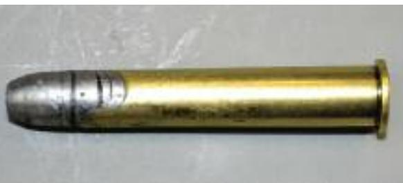
*Not belling the case enough can result in crushing the case.*
