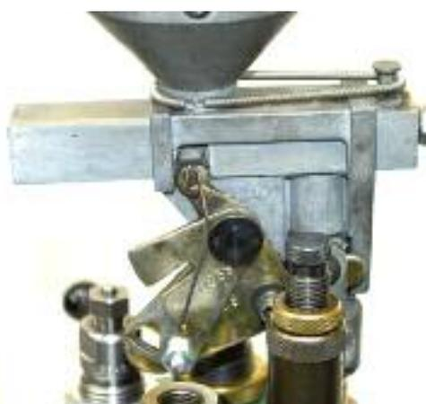
*If you use American Pioneer Powder, you can use a powder measure designed for smokeless powder. I have several Dillons, so I use one. To make it work in this press, you need a return spring and to use a screw and nut to lock the two parts of the bell crank together.*
