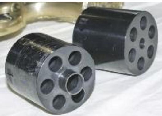
*.38er Colt Navy conversion cylinder (left) with Remington Navy conversion cylinder without gas ring (right). The gas ring on the Colt protects the arbor from fouling*
