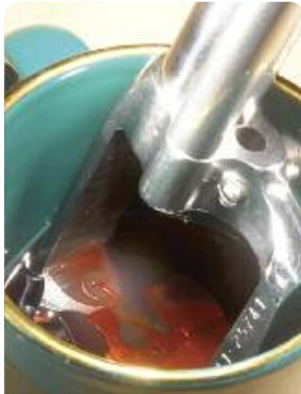
**Soaking In Penetrating Oil Showing Marked Recoil Plate**
