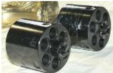
*Recesses for the cartridge rims of Uberti Remington conversion (left) and "flat" breech side of chamber of Uberti Colt conversion (right)*
