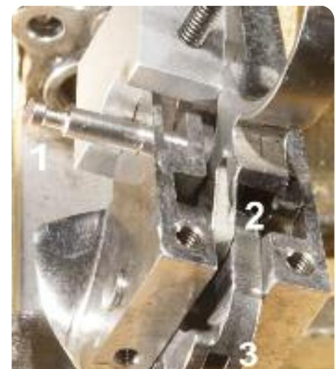
**Partial Removal Of Trigger/ Cylinder Latch Pivot Pin Showing: (1) The Recess In The Pin That Is Held By The Gate Detent Spring, (2) Trigger And Trigger Recess Into Which Trigger Spring Fits, And (3) Hammer Recess For Strut**
