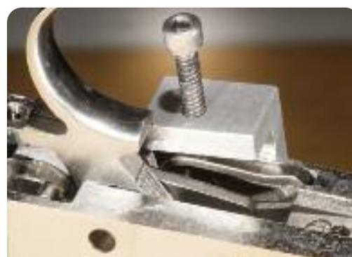
**Gate Spring Clamp Showing Relationship Of Allen Head Screw To Loading Gate Detent Spring**
