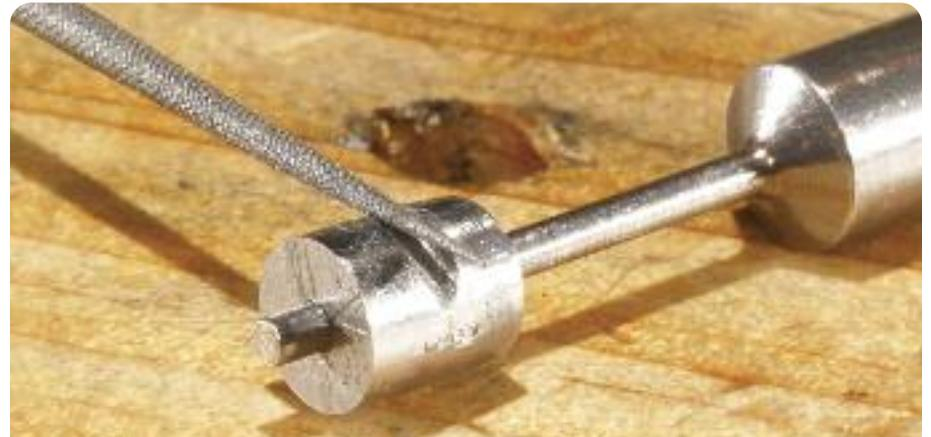
**Figure 8. Filing the Recoil Plate Channel**
