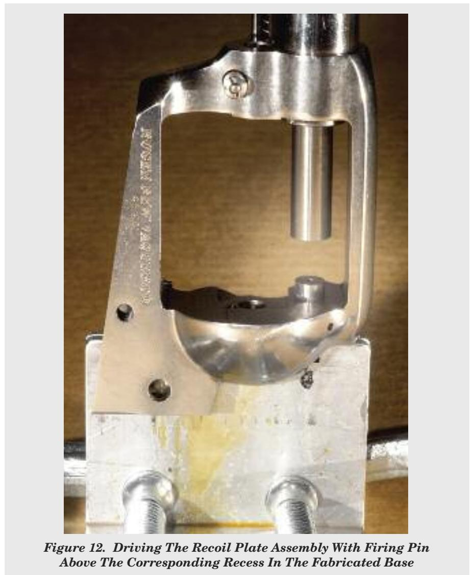
Figure 12. Driving The Recoil Plate Assembly With Firing Pin Above The Corresponding Recess In The Fabricated Base
