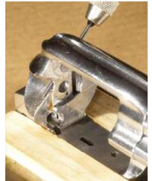
**Figure 10. Follow-Through Drilling Of Existing Recoil Plate Cross Pin Hole To Remove Residue and Cuttings Showing Drill Exposed In The Recoil Plate Recess**
