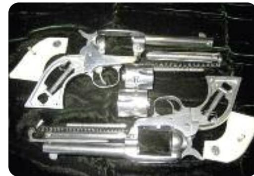
The process to prepare the gun for the new finish is to completely disassemble the firearm. After disassembly, the individual parts are degreased. Preparation for the application involves grit blasting the surfaces of each part to a satin like finish. Then plugging the bore and chambers.
