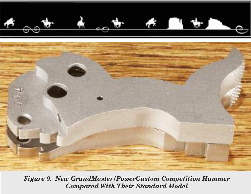
**Figure 9. New GrandMaster/PowerCustom Competition Hammer Compared With Their Standard Model**
