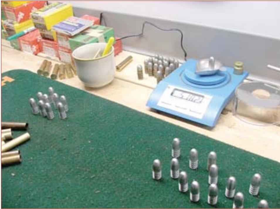
***By weighing each cast bullet, the shooter can weed out ones that are out of spec weight-wise. For real precise shooting, plus or minus a couple grains is okay, but serious long range shooters won't compete with a bullet that is off by more than .2 grains!***
