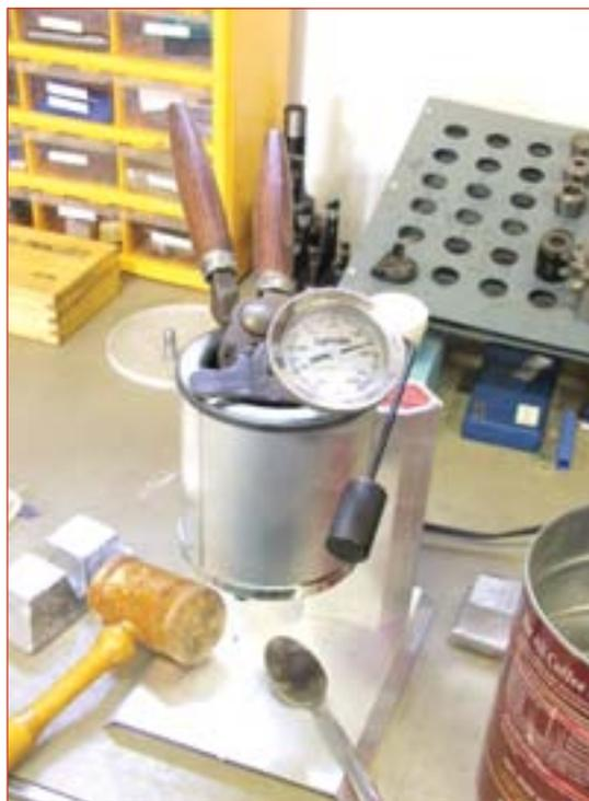
*A thermometer is essential to keep the lead around 800 degrees. The alloy stays together, and the lead flows and cools the best at this temp.*
