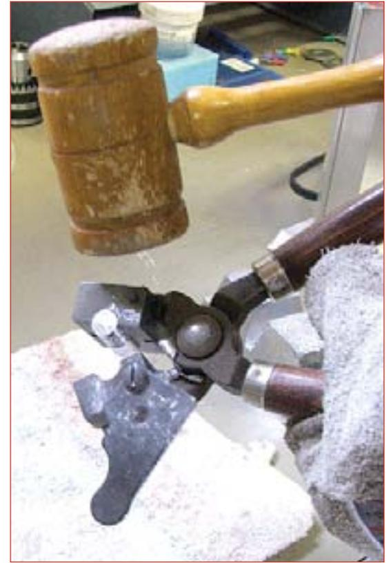
***Tapping out the bullet with a piece of wood or mallet onto a cloth ... the bullets are soft, and a towel or other soft landing keeps them from denting.***
