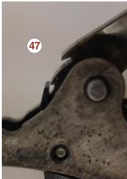
is never used. If you want to go full BOOGIE you can weld up the half cock and grind and polish the front of the hammer to a smooth, clean surface. **Photo 48.**
