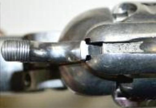
*Original SliX-Shot stainless steel nipples don't allow hammer to seat fully in the frame.*
