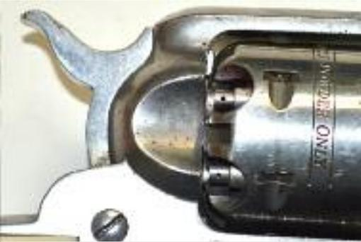
*Original SliX-Shot stainless steel nipples. Both old and new have vent holes in the sides, allowing lighter hammer springs with reliability.*
