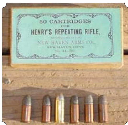
.44 Henry rounds (l-r) — two 215 gr. bullet/25 gr. blackpowder Civil War vintage loads, Tuolumne Lawman's 200 gr. bullet/28 gr. blackpowder Henry duplication load, and three 200 gr. bullet/28 gr. blackpowder Henry Flat loads.
