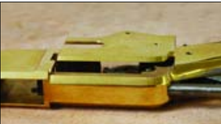
Installation of the side plate. Note the dovetail joint.
