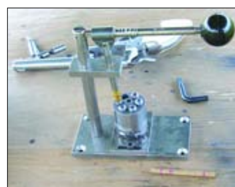
Five balls have been placed in the chambers, and the first one is ready to seat.
