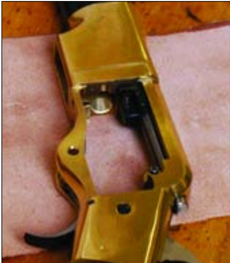
Receiver frame milled out and hand finished.
