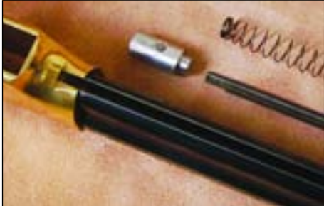
Magazine with follower, magazine spring, and cover.
