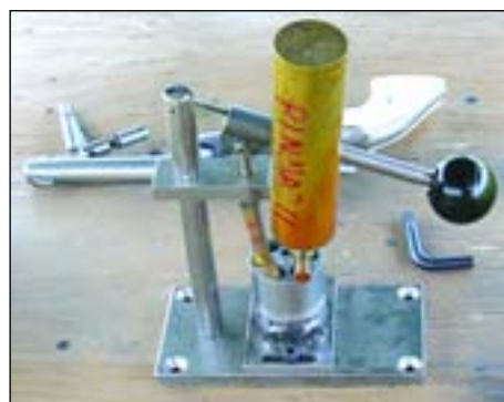
As a dowel marks the last chamber with powder in it, a measured charge is inserted in the next chamber.
