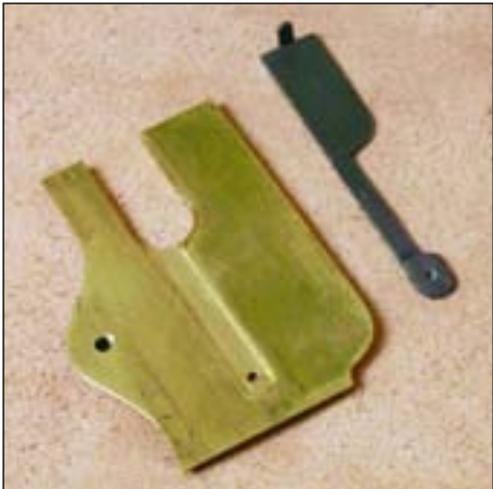
Receiver side plate with spring steel loading gate.
