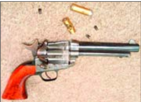
Single Action Revolver, 4 months old. Gives a new meaning to the term “Hand Grenade!” Almost one half of the cylinder is missing, top strap is missing, and ruptured case is seen as well. The bore was clear of any obstructions.
