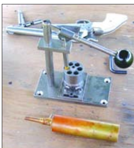
Power Inc.'s Cap and Ball Cylinder Loader ready to insert powder. The Ram holds the cylinder and is in the chamber not to be loaded.
