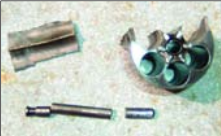
Cylinder after it was removed with a piece of shrapnel created by a piece of the cylinder being blown out. The base pin was in three pieces as the force blew downward causing it to fracture. The operator of the revolver was not injured nor any of the properly positioned and safety equipped spectators or RO. The cartridge case has a bulged primer and rupture in the side. The hole is blown inward, powder is missing, as was the projectile.
