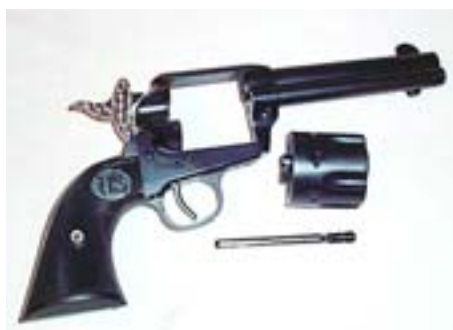
Long Hunter even polished the base pin making for easier cylinder removal and seating. Note the jeweled hammer!
